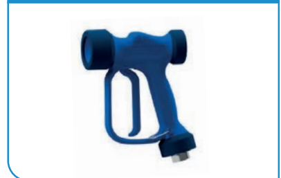
RB65 GUN + SW LOW PRESSURE (FOOD INDUSTRY) ADJUSTABLE 60 L/MIN. 24 BAR
