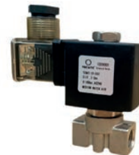
STAINLESS-STEEL SOLENOID VALVE. EPDM. 1/4"NC. 24V AC. MECATIC 0-16 BAR
