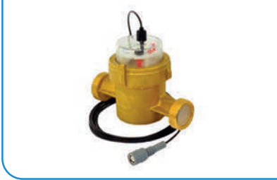
VOLUMETRIC METER DCI-15 1/2" COLD WATER 1 IMPULSE / 1 L
