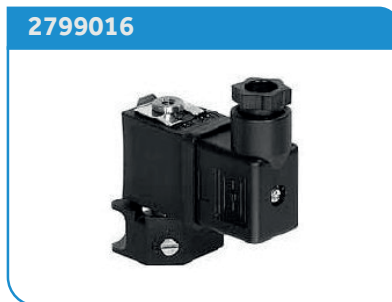
PNEUMATIC SOLENOID VALVE. 0-10BAR. 1/8" 4/2. 24V. DC.
